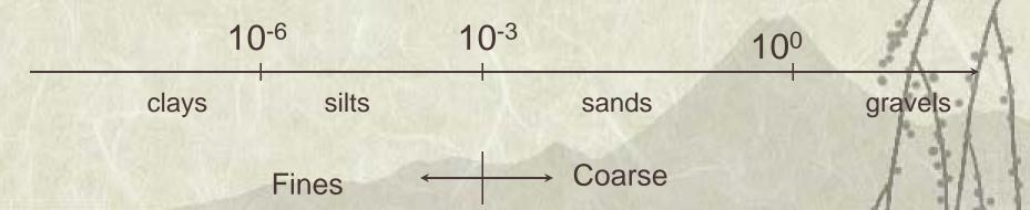
For coarse grain soils,  $k = f(e \text{ or } D_{10})$
