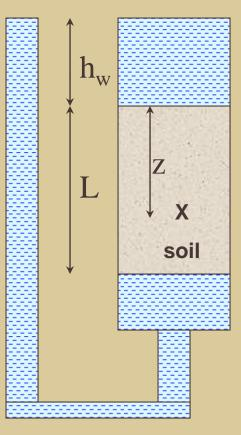
$$\frac{At X}{\sigma_{v}} = \gamma_{w}h_{w} + \gamma_{sat}z$$
