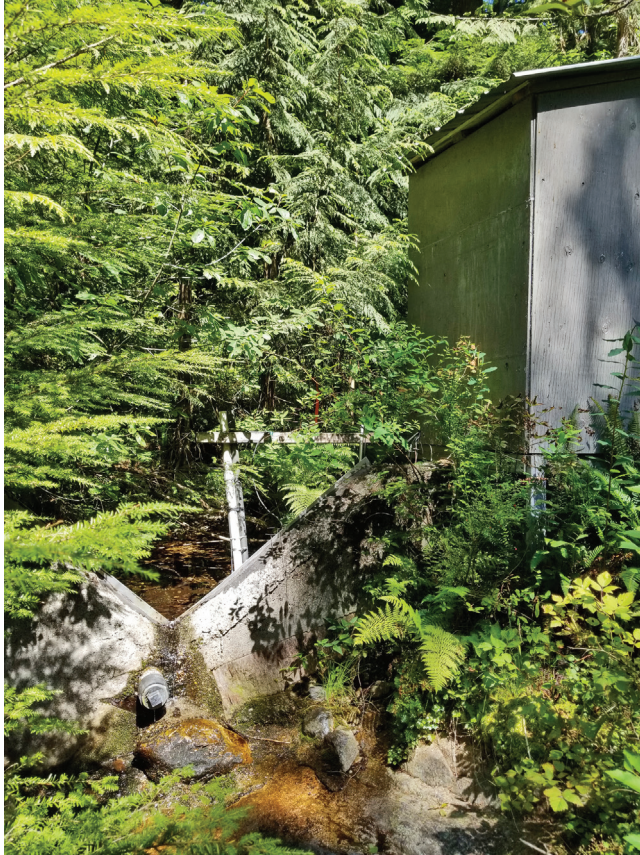
Figure 1.2 A V-notch weir used to measure the height of the water surface; in this case, from a very small watershed. Water slows in the pond that was dammed just upstream of the weir, and the height of the water can be recorded on a pressure transducer, which measures the elevation of the water surface above it. Higher flows result in deeper water in the pond. The actual discharge in L/s still needs to be calibrated through a rating curve that relates the height of water to the flow, and this can be done by using a couple of methods, based on depth and current velocity profiles, or salt-dilution gauging. The calibration depends on getting a regression of discharge against the pressure reading. In very simple systems, there may be a staff gauge, which is often a big ruler that someone must read directly for water depth, but still needs calibration.
