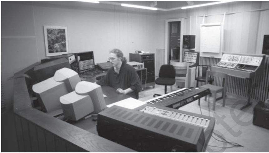
Figure 6.7 Control rooms usually need to have short reverberation times. It is often necessary to remove undesirable reflections by sound absorption or sound scattering. School of Music, Gothenburg, Sweden. (Photo by Mendel Kleiner.)
