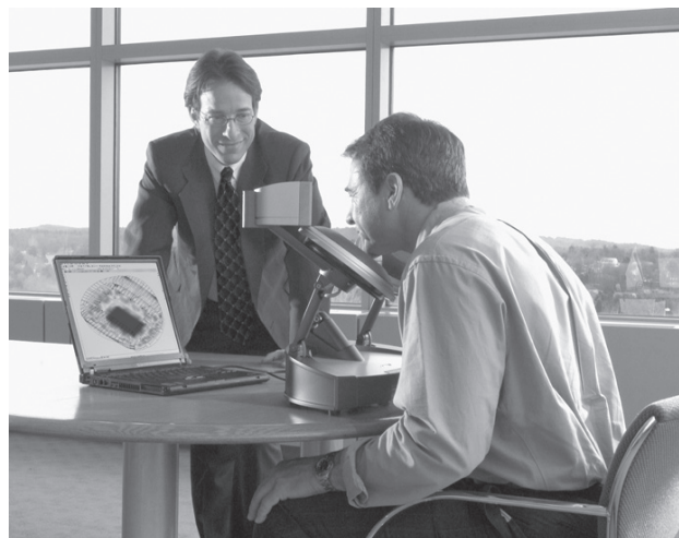
Figure 6.23 The Bose Auditioner® system is a commercial system for auralization using CAD. The binaural room impulse responses are convolved with music or speech so that it is possible to listen to a simulation of what it would be like to listen in the actual room being simulated. Crosstalk cancellation is used to render the binaural signals in this setup (photo courtesy of Bose Corporation).
