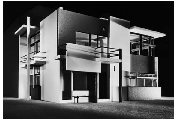
2-13 Conceptual model of a building, scale 1:100. Materials: various types of cardboard. Example of a successful preliminary model used to design a presentation model.
